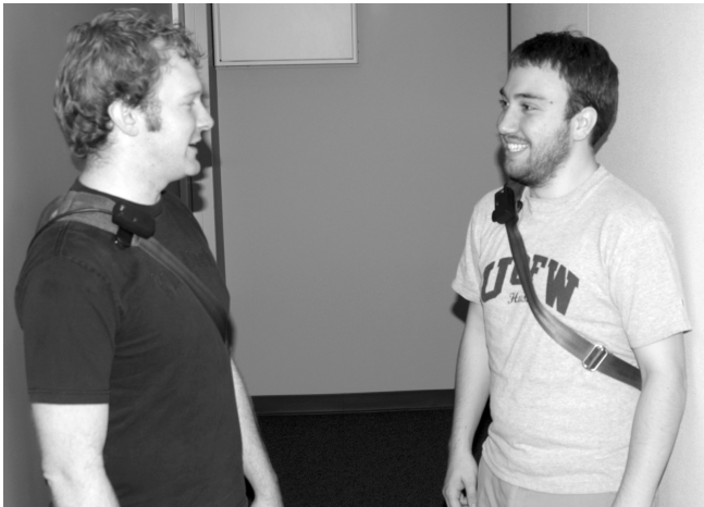
Figure 5: Two people wearing our portable recording equipment. The sensing unit is at their right shoulders.
